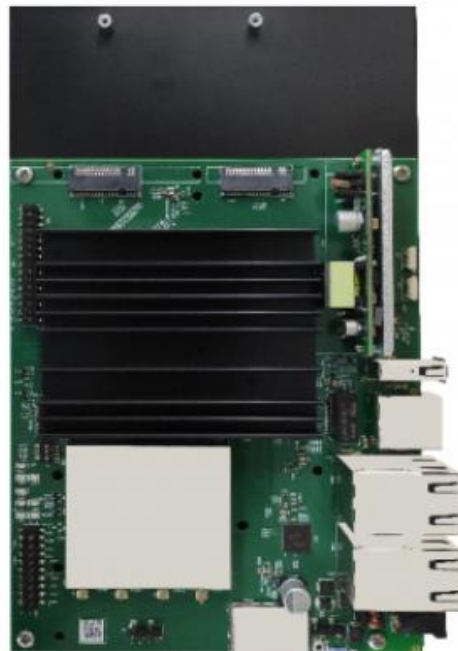
Figure 3: Cost Effective 5G Supported WiFi 6 Board
