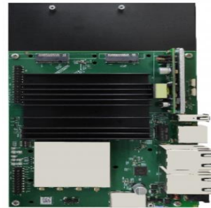
Figure 3: Cost Effective 5G Supported WiFi 6 Board
